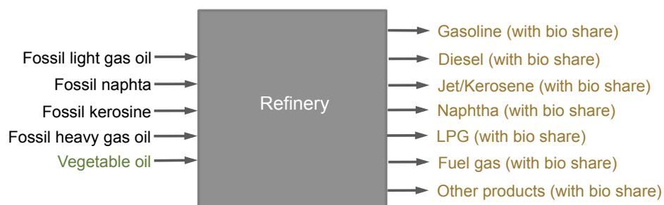
Figure 1: Co-processing of bio-based and fossil feedstocks in a mineral oil refinery
