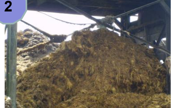
EFB shredded in hammer mill
