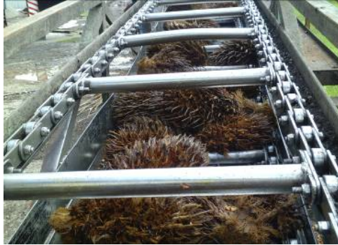
EFB transport with EFB conveyor
