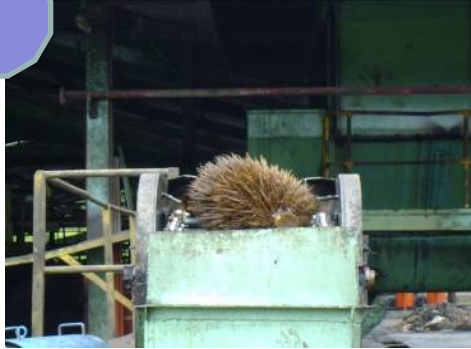
EFB transport with EFB conveyor
