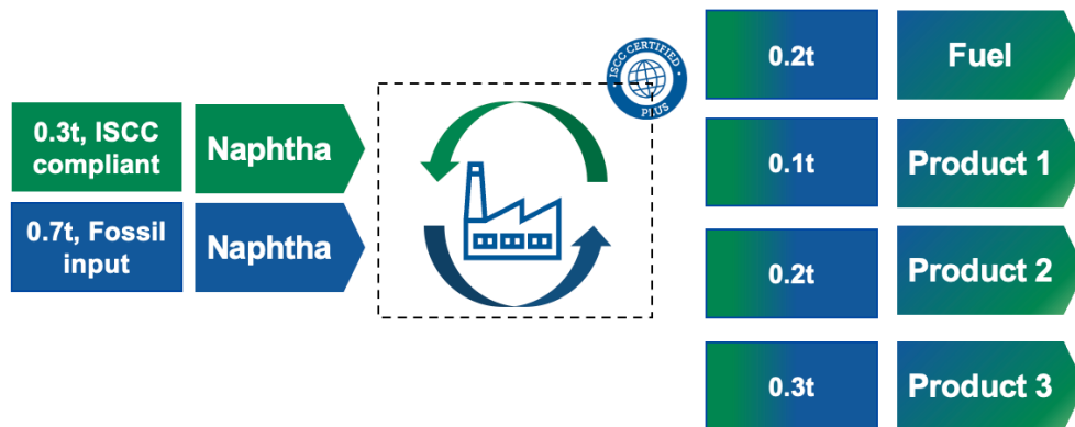
Figure 2: Numeric representation of the steam cracker setup of ISCC PLUS certified and fossil-based Naphtha over a mass balance period.
